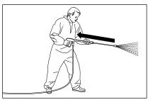
When using high pressure water for cleaning, make sure that there is a clearly noticeable recoil effect on the lance. Therefore ensure a firm footing (see technical data).
