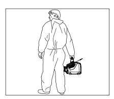
1. Carry the K 1050 P to its place of operation. When parking the high pressure cleaner make sure that the four rubber buffers stand on a safe support.
